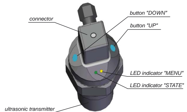
Full view of ultrasonic level meter
