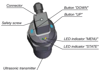
Fig. 16: Full view of ultrasonic level meter
