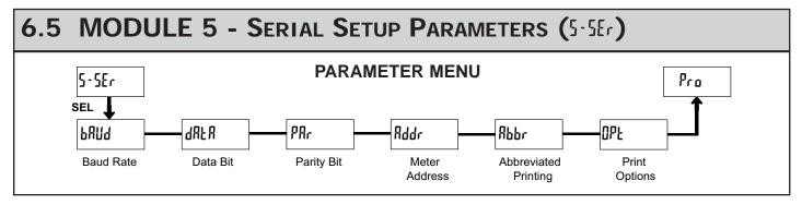
The Serial Setup Parameters are only active when one of the optional serial communications/programming cards is installed in the meter. Refer to the CUB5COM bulletin for details and setup for the CUB5 RS232 or RS485 serial communications. Refer to the CUB5USB bulletin for details on the CUB5 USB programming and programming requirements.
