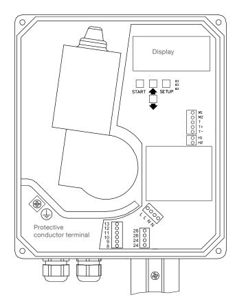
Internal terminals for motor and heater
