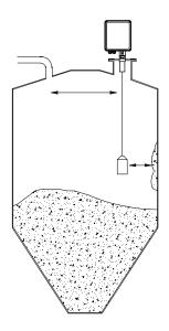
Measurement during filling of the silo
