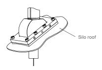
Flange plate outside dimensions: Width x Heigth: 120mm x 180mm (4.7"x7.1")
