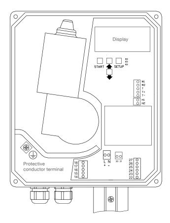
Internal terminals for motor and heater
