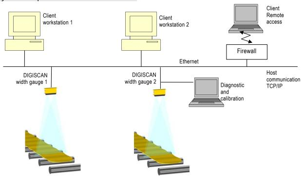
The DigiScan Width Gauge sensor captures all the edge data and computes width and centreline. This information along with other I/O and alarm data is passed on to a number of computers through an Ethernet communication channel. A Windows based workstation computer acquires the width measurements and centre line deviations from the DigiScan sensor, using TCP/IP high speed link.
