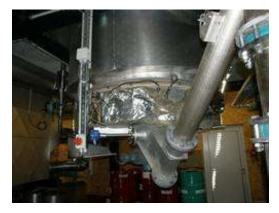
A manufacturer of wood gasifier systems had the application of an empty detection in a reactor vessel. The sensor should reliably detect ash. The process temperature range is up to 250 ° C. The application is sticky and very dusty. The sensor should therefore be robust, insensitive but sensitive enough to guarantee a reliable empty detection of the reactor.
