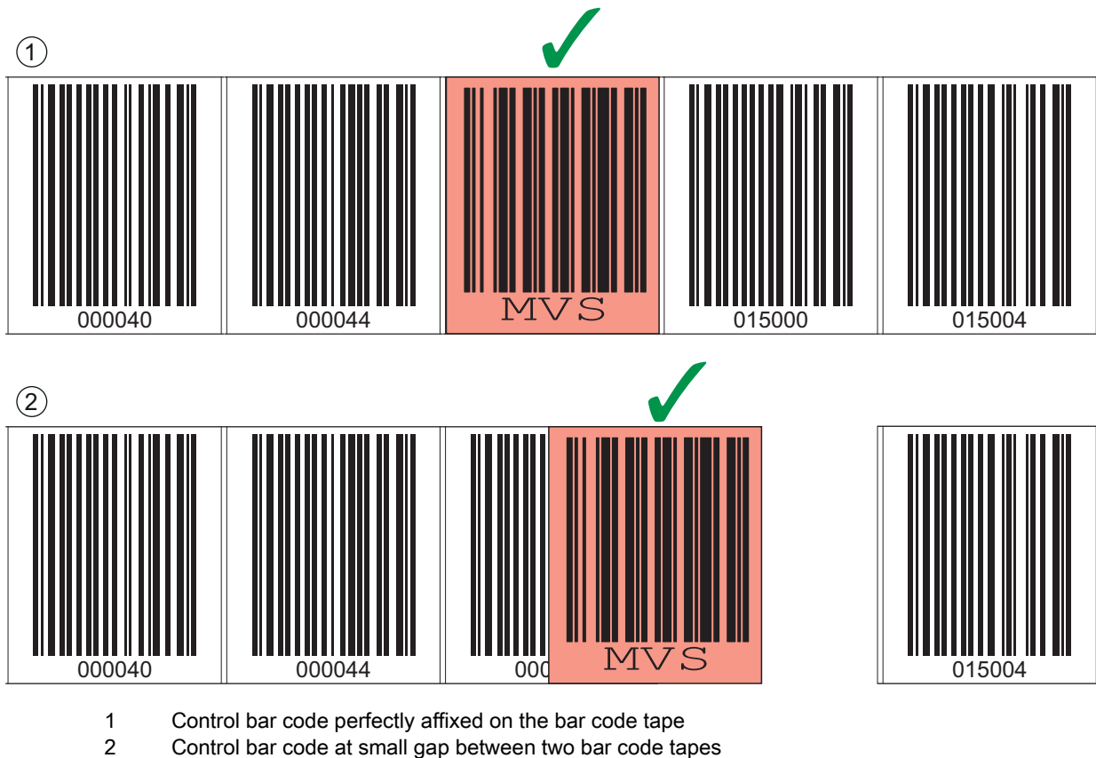
Figure 3.11: Correct positioning of the control bar code
