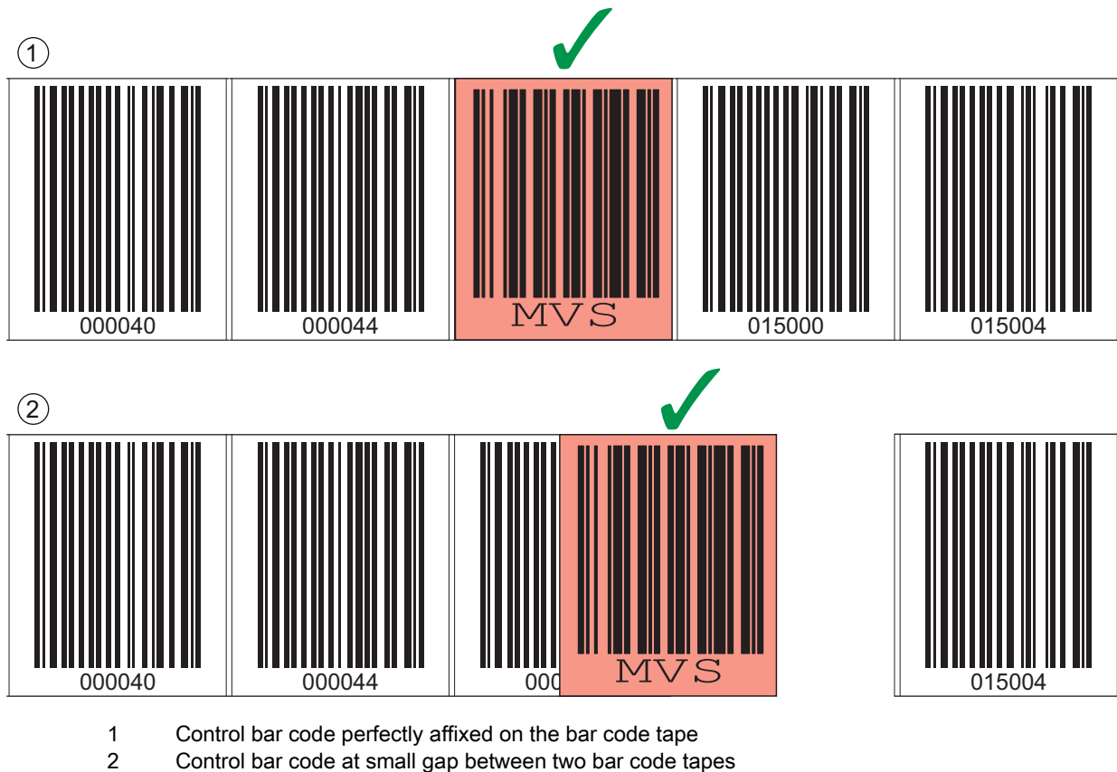
Figure 3.13: Correct positioning of the control bar code
