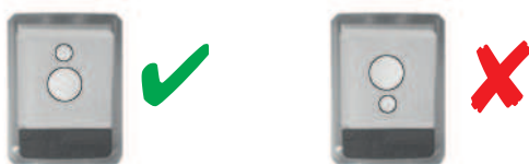
Fig. 6.8: Orientation of the diffuser foil
