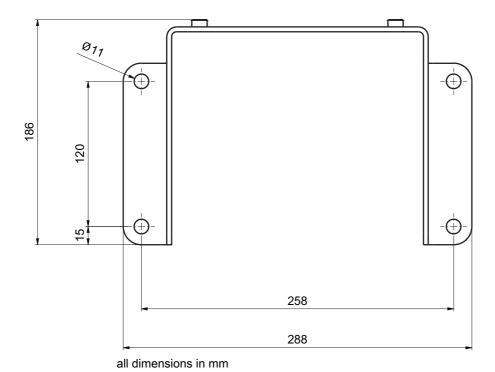
Figure 15.6: Mounting bracket BTF815M
