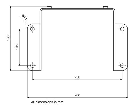
Figure 15.7: Mounting bracket BTF830M
