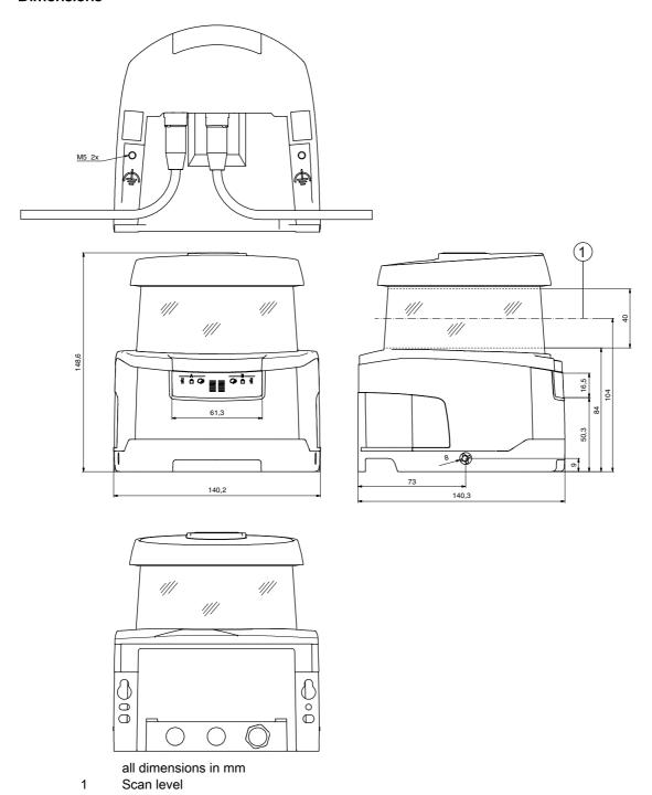
Figure 15.1: Dimensions safety laser scanner with connection unit
