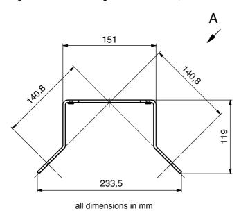
Figure 15.11: Mounting bracket BT856M
