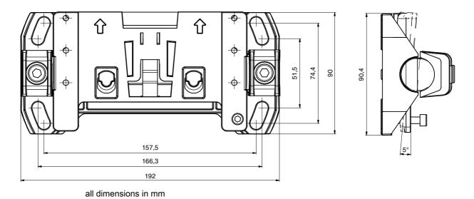
Figure 15.5: Mounting system BTU800M
