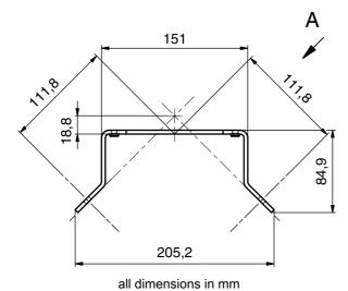
Figure 15.9: Mounting bracket BT840M
