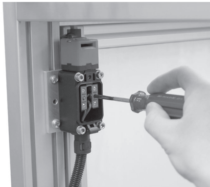
Figure 7.5: Connection example S200-M3C1-M20
