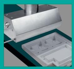
Cleaning (e.g. PCBs) with ionized air and rotating nozzles with a simultaneous vacuum aspiration
