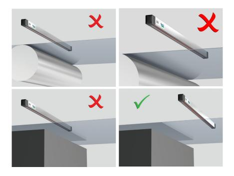
3. Avoid proximity to earthed parts of machinery as this will distort the corona and reduce its efficiency.
