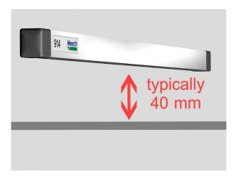
Mounting of the bar is by 20mm M4 studs mounted at the rear of the bar. The chassis of the bar is electrically connected to ground on the power unit via the flexible armoured conduit. However, it is good practice to provide a secondary grounding through the fixing points where practical.
