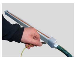
Holding the wire insulation, approach any of the bar emitter pins with the bare end of the wire.
