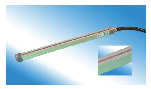
The Meech Model 914EX has been designed to meet the most arduous of static elimination problems. The special resistive coupling of its emitter pins renders them shockless, whilst giving powerful static neutralisation performance. This enables the Bar to eliminate very high static charges on high speed webs and at longer ranges than has been previously possible.
