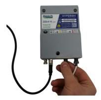
12. Using a high voltage probe ( RS type 610 281 ) and meter ( RS type 610 950 ) measure the voltage on each of the output sockets. The reading should be at minimum power 4kV and at maximum power 8 kV
