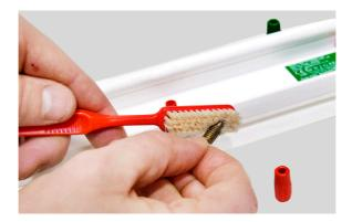
lonisers will need periodic wiping to clean grey deposits from the surface of the bar. A cloth moistened with a small amount of IPA or methylated spirits is recommended.
