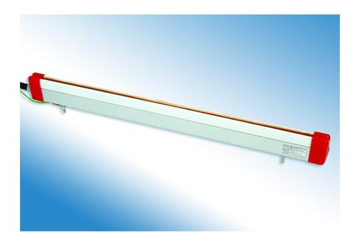
The Meech Model 915EX has been designed for use on the most arduous static elimination problems. The special resistive coupling of its emitter pins renders them shockless, whilst giving powerful static neutralisation performance. This enables the bar to eliminate very high static charges on high speed webs and at longer ranges than has previously been possible.
