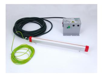
The Power Unit converts the electrical supply into a high voltage, low amperage output. This output energy is transferred to the 915EX bar by the HT cable.
