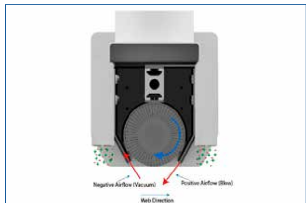
RoClean-C Web Cleaner (cross section of airflow and brush direction)
